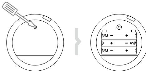
To insert or replace batteries, unscrew the screw and prise the plate open. Load the batteries into the compartment and screw the plate back. If the batteries are flat, charge them with a recommended charger by connecting it to the USB port of the soothing device.
