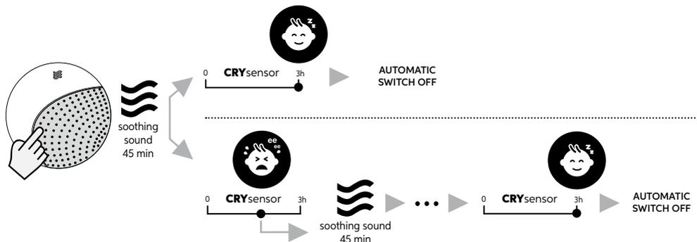
To turn the device on or off, press the top of the device briefly once. It will gradually automatically reduce the sound volume and automatically switches to the 3-hour **CRY**sensor stand-by mode.
